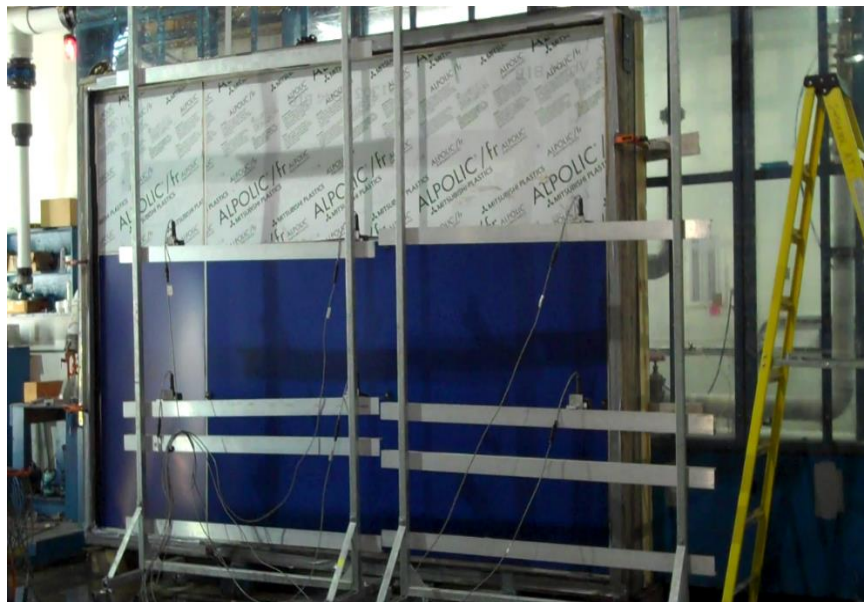
Photo No. 2 Linear Transducer Setup
